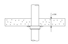
5. One collar on the bottom side of the floor is sufficient for floor penetrations.
