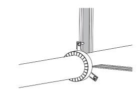
4. The MG2-A may be fixed by universal screws (M6) or by threaded rods, washers and bolts.
