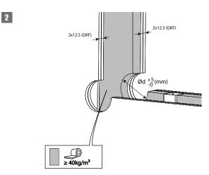
2. Insulate the wall and finish with two gypsum plasterboards type F.
