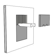
5. Put the second stone wool board of min. 50mm thickness around the pipes. Avoid the joints from coinciding. Apply endothermic coating (type PROMASTOP-E) on the lateral sides, as well as on the joints.
