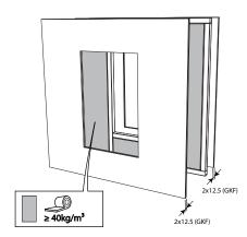
1. Provide an installation opening of maximally 1000 x 600 mm.
