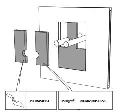
3. Place the plastic pipe(s). The distances between the pipes and the edges of the seal are min. 100 mm.
