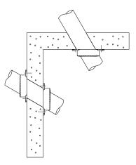
6. For oblique penetrations till 30°, choose the collar with dimensions as close as possible to the outside diameter of the pipe. See the classification report on www.rft.eu for an overview of the classifications.
