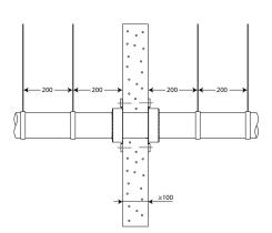
3. Reinforced concrete: place expander bolts in the pre-drilled holes  $\emptyset$  6mm and fasten them. Aerated concrete: fix with universal M6 screws.
